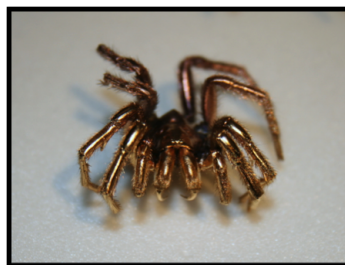
Figure 3: A spider sputter-coated in gold, in preparation for SEM imaging.
